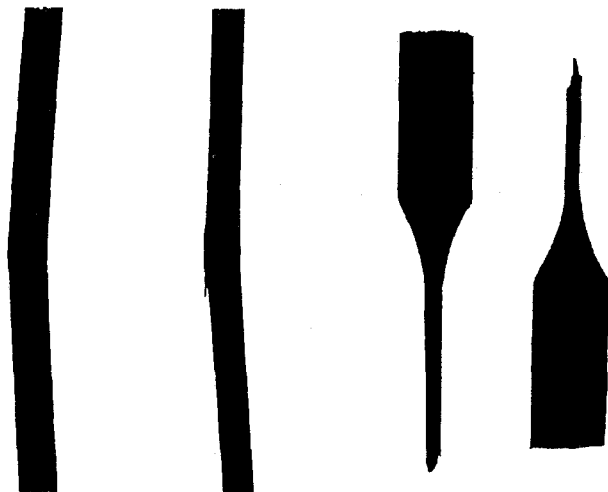
Figure 1 Geometry and typical fracture behaviour of stressed samples in the bending and tensile test.
